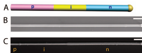
Figure 1. Scheme and structural characterization of axial p-i-n SiNWs. (A) Schematic of an axially modulated p-i-n SiNW. Growth is mediated with Au catalyst (gold-colored hemisphere) in a sequence beginning with p -, i -, and ending with n -regions. (B) SEM image of a uniform p-i-n axial SiNW with Au catalyst ( d = 250 nm) visible on the right-end. (C) SEM images of a p-i-n axial NW after selective wet etching. The p - and i -type Si regions have faster etching rates than the n -type region (see text for more details). Scale bars are 1 \mu m.
