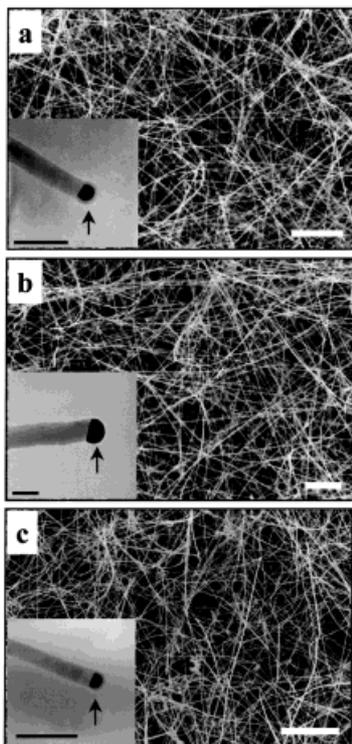
Fig. 2. FE-SEM images of a) GaAs, b) GaP, and c) GaAs<sub>0.6</sub>P<sub>0.4</sub> nanowires prepared by LCG (the scale bars are 2 μm). The respective insets are TEM images of GaAs, GaP, and GaAs<sub>0.6</sub>P<sub>0.4</sub> nanowires (the scale bars are all 50 nm). The high contrast (dark) features correspond to the solidified nanocluster catalysts.
