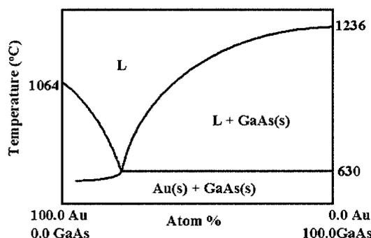
Fig. 1. Pseudobinary phase diagram for Au and GaAs. The liquid Au–Ga–As component is represented as L.
