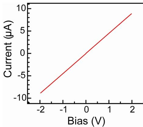
**Figure S1.** Current-voltage data recorded between two Ni contacts for a Si/a-Si NW. The linear behavior confirms that the Ni contacts to the NW are ohmic.
