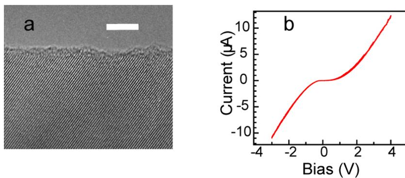
**Figure S2.** Si NW x M NW control devices. **a**, HRTEM image of a Si NW used in these experiments without the a-Si shell layer. Scale bar is 5 nm. **b**, Current-voltage data recorded between the ohmic (Ni) contact to the Si NW and the Ag NW electrode for a representative device. No switching was observed.
