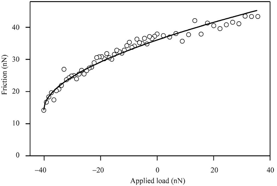
**Figure 2.** Friction force *versus* applied load curve (○) for a CH<sub>3</sub>-terminated tip and sample in water. The concave shape of the curve is consistent with the non-linear dependence of the contact area on external load predicted by the JKR model, equation (1) (—). Absolute friction values are reported here without the adjustment for the contact stiffness in the detector calibration (they are about a factor of 1.5 higher than the actual values).
