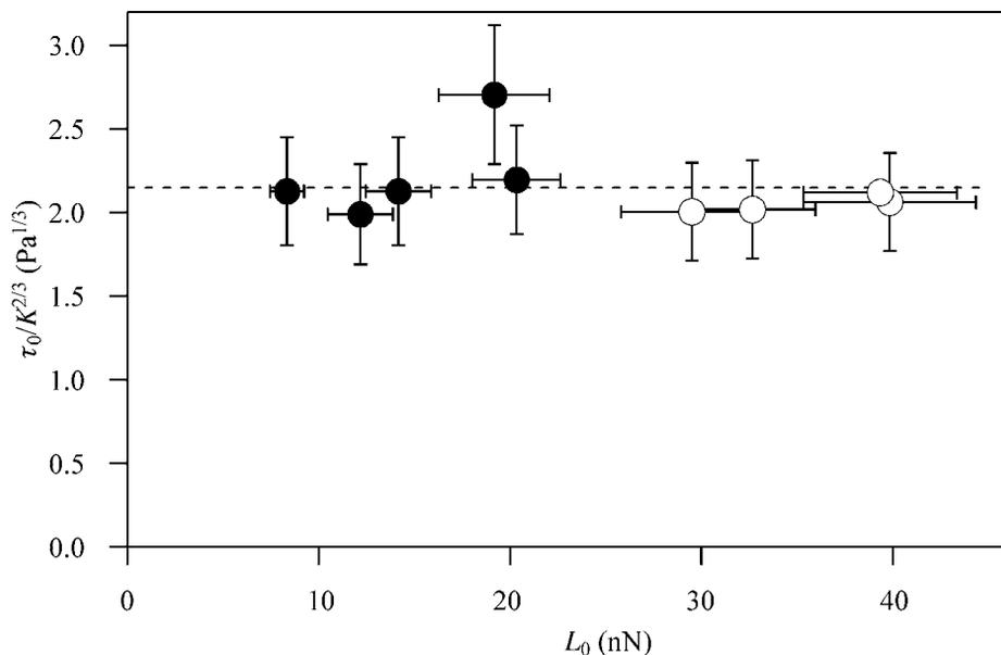
**Figure 4.** Interfacial shear strength,  $\tau_0$ , normalized by the elastic constant,  $K^{2/3}$ , versus the force of adhesion measured simultaneously from the curves of the type shown in Fig. 3. Error bars represent standard deviations from the mean values found in the analysis of approximately 100 single curves. Closed and open symbols represent two different experiments.
