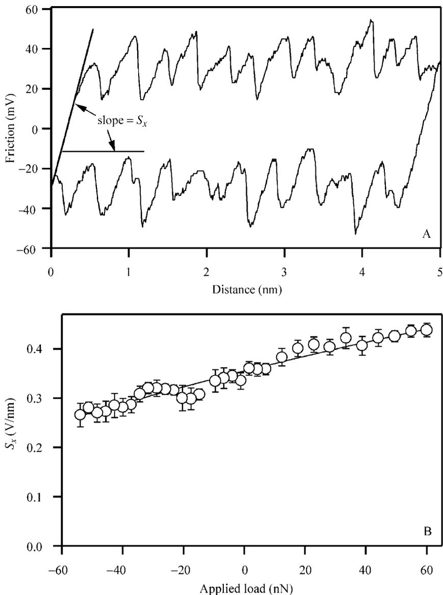
**Figure 1.** (A) Determination of the lateral sensitivity ( $S_x$ ) of the photodiode detector from atomic stick–slip friction loops on mica. (B) Dependence of the lateral sensitivity determined in (A) on the external load applied to the tip.
