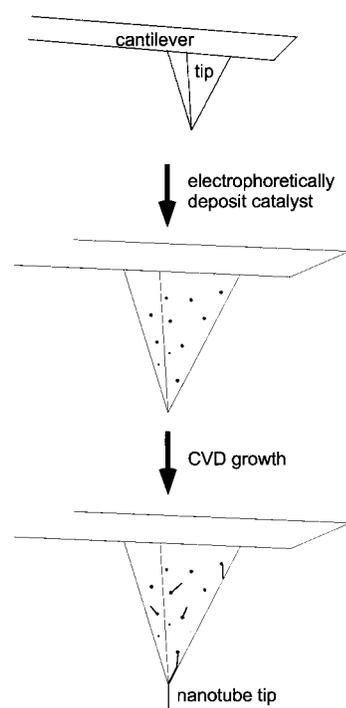
Figure 1. Overview of the approach used to prepare SWNT tips.
