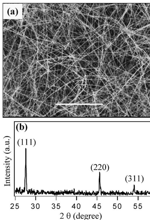
FIG. 1. (a) FE-SEM image of GaAs nanowires obtained from a  $(\text{GaAs})_{0.95}\text{Au}_{0.05}$  target by LCG. The scale bar corresponds to  $5 \mu\text{m}$ . (b) XRD pattern obtained from a bulk sample of GaAs nanowires.
