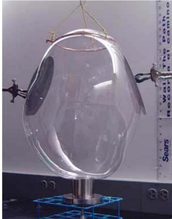
*The blown bubble film (bubble diameter 35 cm; height 50 cm) has coated the surface of two 150-mm silicon wafers. The range of the ruler behind the bubble is 0–23 inches (0-58.4 cm). (Image: Cao/Lieber)*
