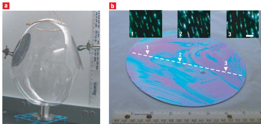
**Figure 1** Blown-film extrusion is a promising technique for making nanocomposite films. **a**, A photograph showing the transfer of a bubble containing silicon nanowires suspended in a polymer to a pair of 150 mm silicon wafers. **b**, Image of a 200 mm silicon wafer onto which single-walled nanotubes have been transferred. The insets are dark-field images showing the alignment of the nanotubes at three different locations on the wafer. (See ref. 1 for full details.)
