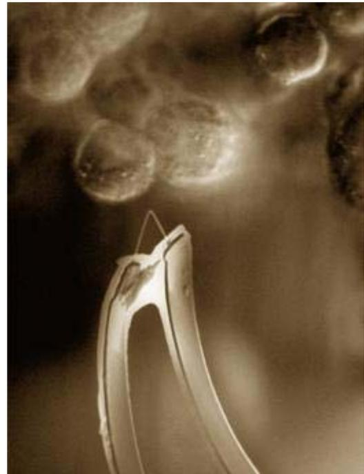
A nanoprobe has been used to measure the electrical activity of a cell.
