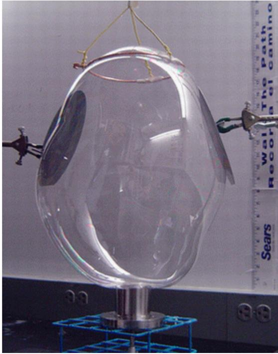
A blown-bubble film (bubble diameter is 35 cm, height is 50 cm) that has coated the surface of two silicon wafers. Credit: Charles Lieber, et al.
