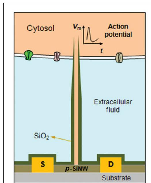
A schematic diagram of a cell coupled to the branched nanotube field-effect transistor during an action potential  $V_m$ . S and D indicate source and drain electrodes. Reproduced with permission from *Nature Nanotech.*, DOI: 10.1038/NNANO.2011.223. © 2011 Macmillan Publishers Ltd.
