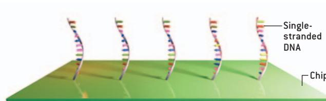
1 Single DNA strands are attached to a silicon chip. They encode all possible values of the variables in an equation that the researchers want to solve.
