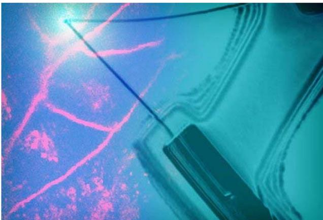
**Nano-FET** A new nanoprobe can be used to measure the electrical activity of a cell. *Courtesy of Charles Lieber*
