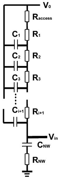
Fig. S5. Device bandwidth circuit model. Equivalent circuit used for the BIT-FET device bandwidth model.
