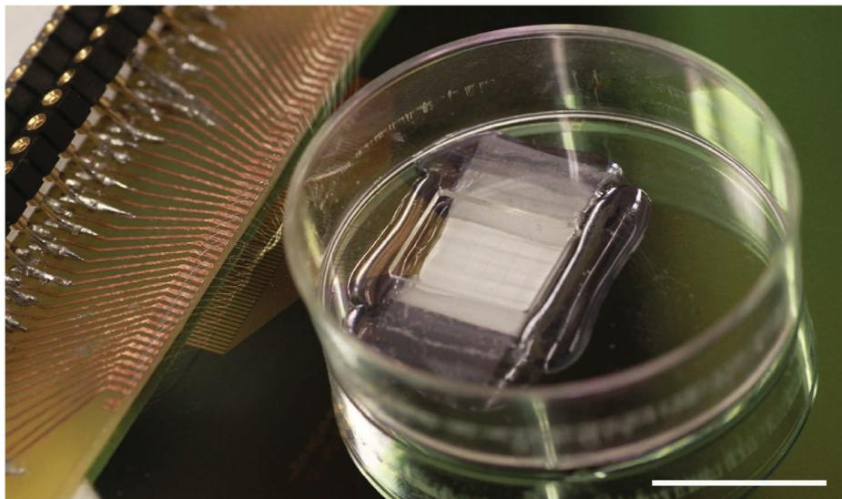
**Figure 1** | Photograph of the 3D scaffold attached to a modified Petri dish. The input-output connections of the chip are visible on the left. Scale bar, 1 cm. Reproduced from the Supplementary Information for ref. 3, Nature Publishing Group.
