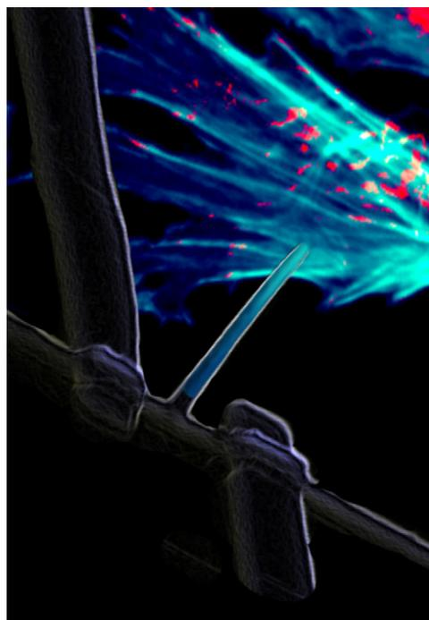
**Figure 2** A false color scanning electron micrograph of a branched intracellular nanotube field-effect transistor (BIT-FET) device overlaid with an image of a cluster of cardiomyocyte cells illustrating how intracellular action potentials are recorded by the device. (Credit: Xiaojie Duan and Brian Timko, Harvard University and Opusdesign.)
