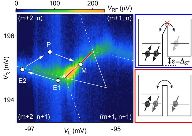
Figure S1: Reversed  $T_1$  pulse sequence.  $V_{RF}$  at the measurement point  $M = (V_L, V_R)$  of the reversed, cyclical Pauli blockade pulse sequence, indicated by white arrows. The pulse diagram has been scaled by a factor of 0.8 to fit on the plot. Dashed lines estimate changes in double dot hole occupancy  $(m, n)$ , where  $m$  ( $n$ ) denotes the occupancy of the left (right) dot. Large solid triangle outlines the region over which direct interdot charge transitions can occur.
