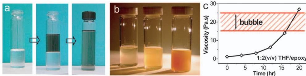
**Fig. 2** Bubble solution preparation. (a) Mixing of NTs dispersed in THF with epoxy to make a uniform solution. (b) Different concentration SiNW–epoxy solutions: From left to right are 0.01, 0.03, 0.15 wt%, respectively. (c) Viscosity *versus* curing time for an epoxy solution, where the range suitable for bubble expansion is highlighted (hatched area).
