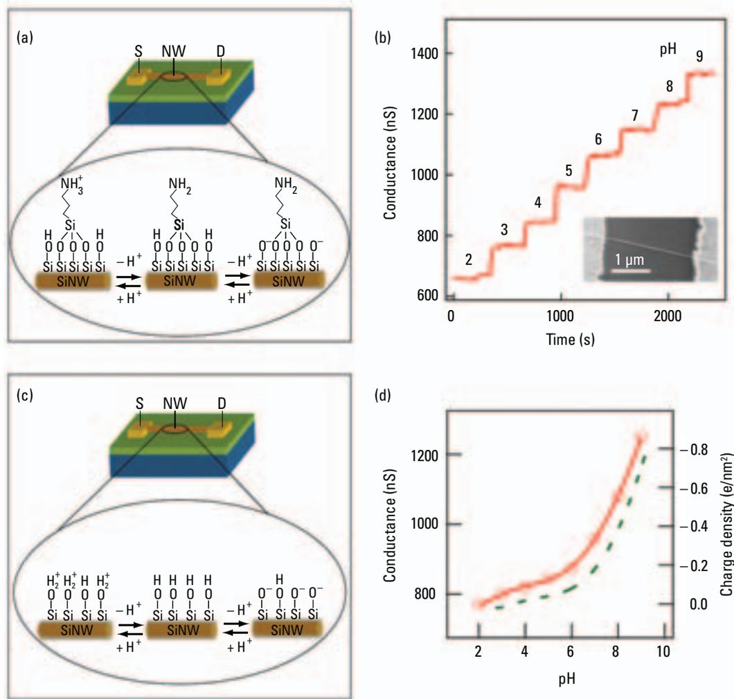
**FIGURE 2.** NW pH sensors.
