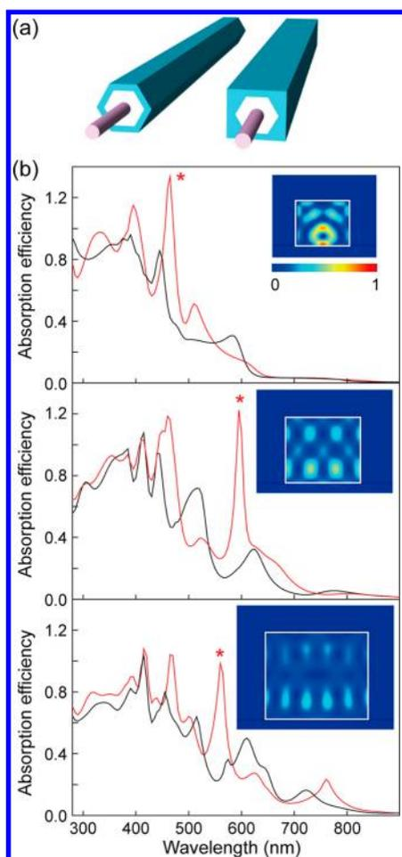
**Figure 4.** (a) Schematics of p/i/n Si NWs with hexagonal (left) and rectangular (right) cross-sectional geometry. (b) TE absorption spectra of hexagonal (solid black) and rectangular (solid red) NWs with heights of 160 (top), 240 (middle), and 320 nm (bottom). The inset shows the absorption profile of the peak marked by \* in each spectrum.
